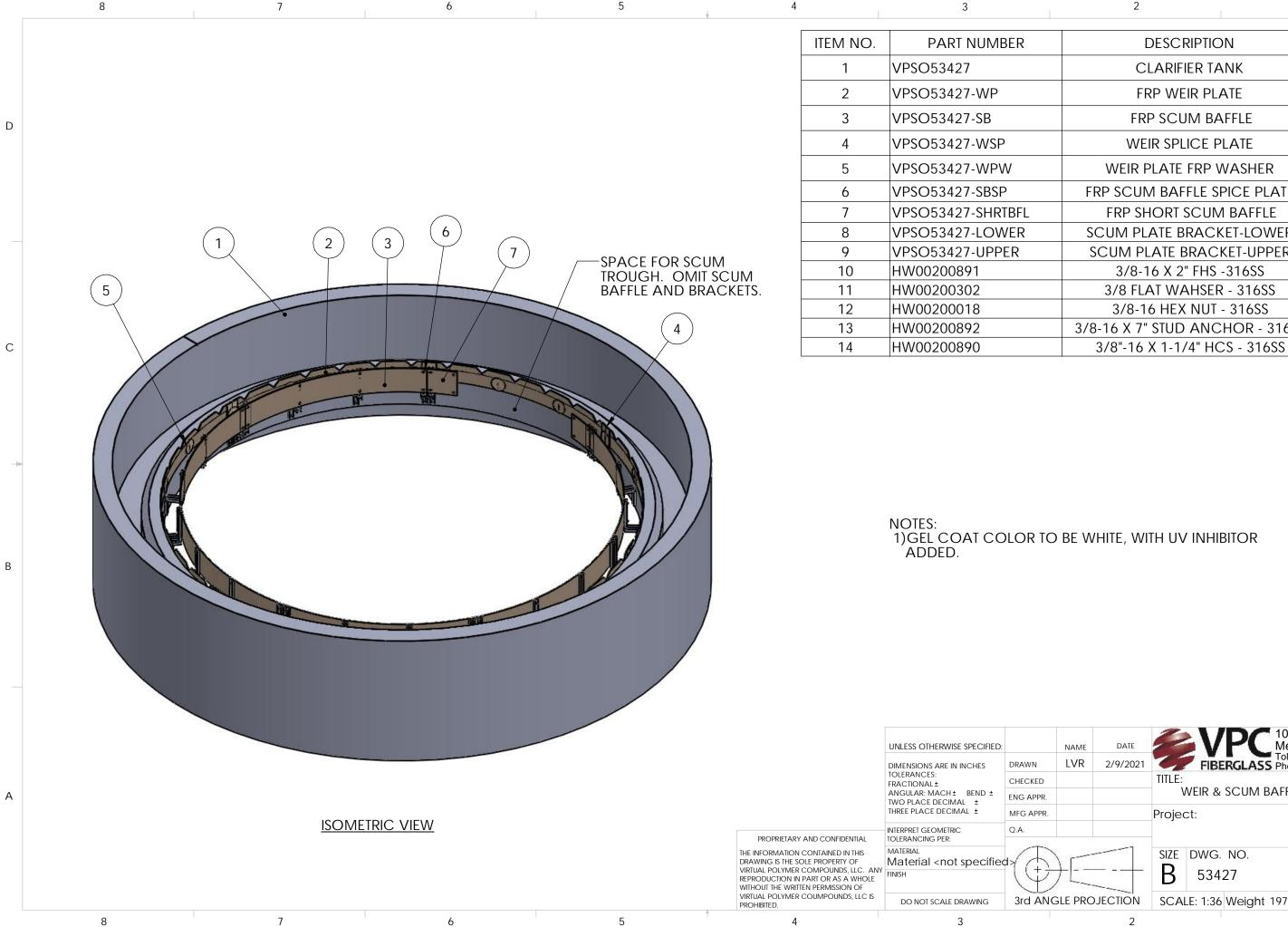
QTY. 1 7 6 7 WEIR PLATE FRP WASHER 21 7 FRP SCUM BAFFLE SPICE PLATE 2 FRP SHORT SCUM BAFFLE SCUM PLATE BRACKET-LOWER 26 26 SCUM PLATE BRACKET-UPPER 52 3/8-16 X 2" FHS -316SS 104 3/8 FLAT WAHSER - 316SS 104 3/8-16 HEX NUT - 316SS 3/8-16 X 7" STUD ANCHOR - 316SS 73 52
